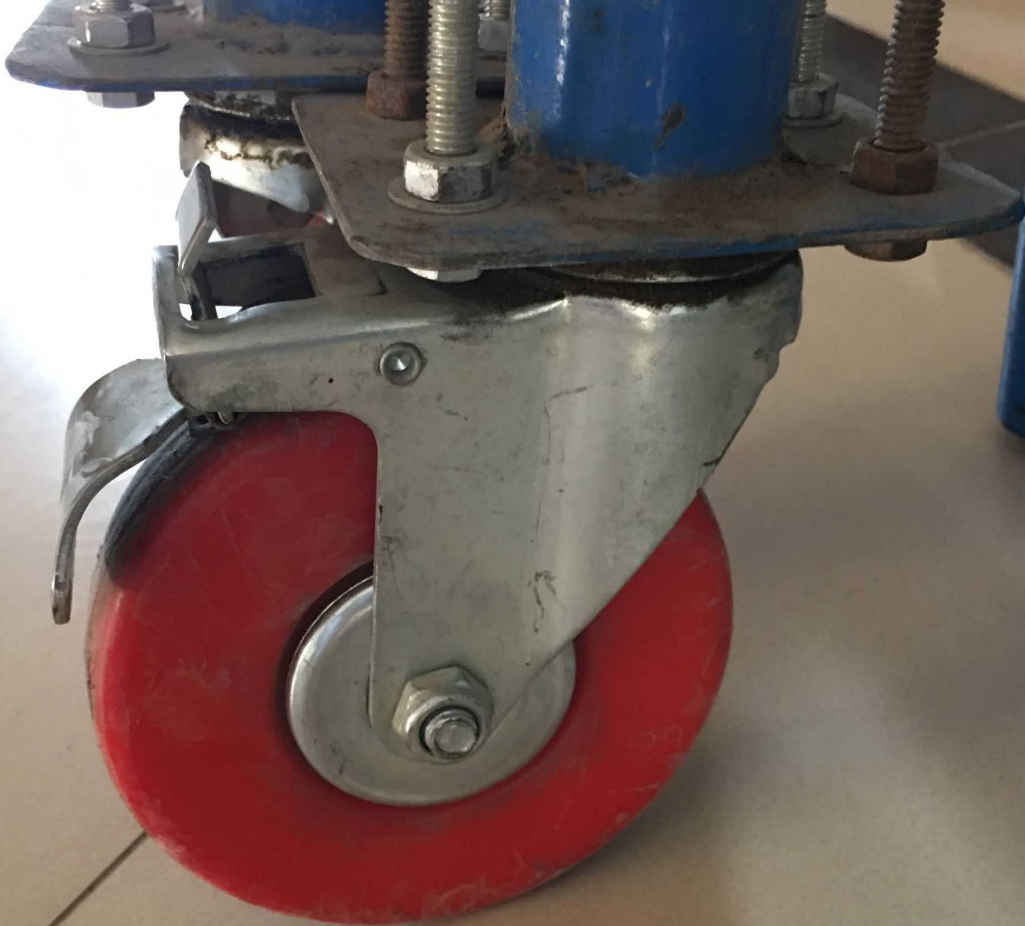
Mini 5" Diameter heavy duty Caster wheel with locking arrangement. Connected with steel frame through bolt (A sample picture is shown above)
