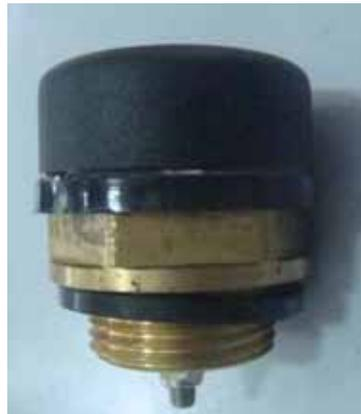
Figure 8 : Pressure Relief Device (PRD) without contacts
