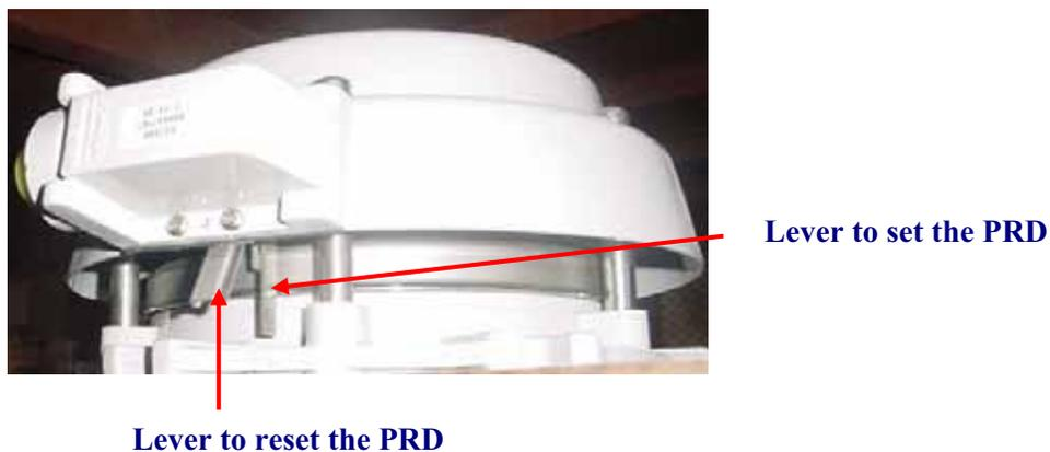
**Figure 10 : Set and Reset levers of PRD**
