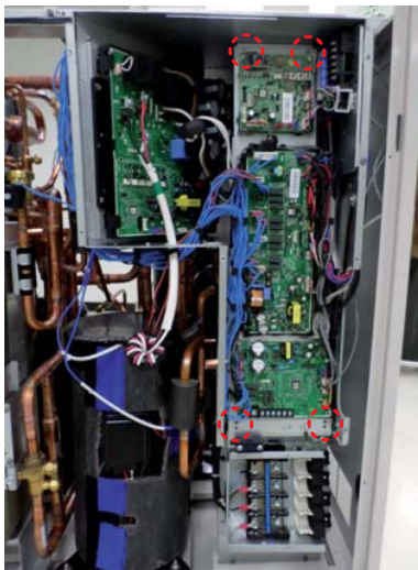
► Separate double layer structure of C/Box after remove 3 screws and connector.
