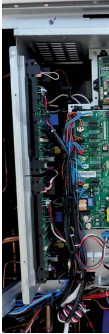
► Comp Wire fix by Holder Wire.
