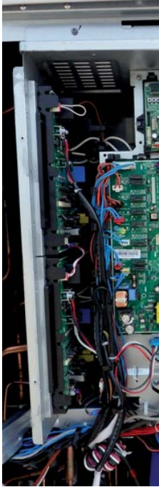
► Comp Wire fix by Holder Wire.
